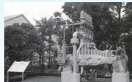
A 6,000 kW back-pressure turbine displayed at the entrance to the Mitsubishi Heavy Industries Nagasaki Shipyard & Machinery Works
